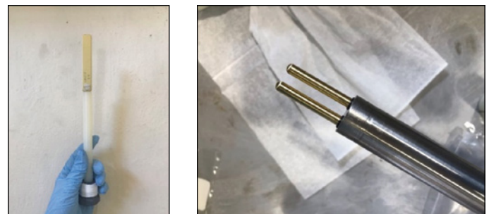
Figure 2. Examples of metal coupon (left) and linear polarization resistance electrodes (right).
